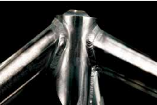
Precision hand welding is elevated to an art form in this engine mount truss structure.
