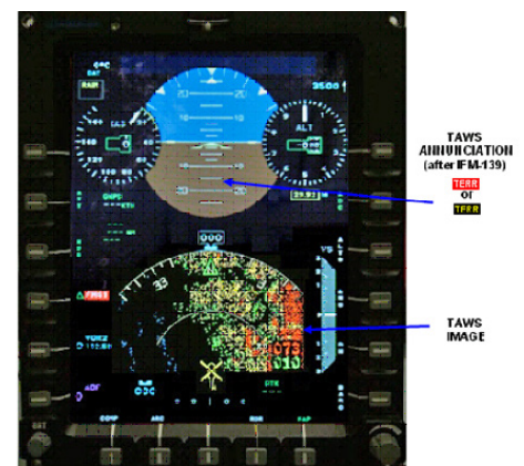
TAWS displayed as HSI underlay on PFD
