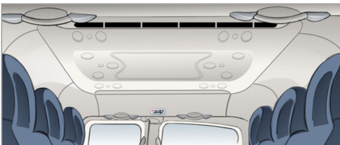
Standard headliner with slotted air vents.
