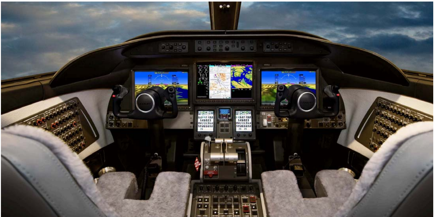
The Learjet 75 is equipped with the latest Garmin G5000 integrated flight deck.
